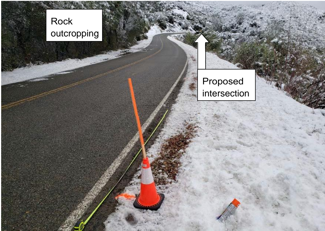
Figure 4 - Sight distance measurement to the right of the intersection.
