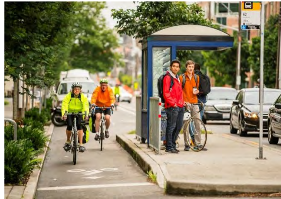
Figure 23: Separated bike lane protected by transit boarding island.
