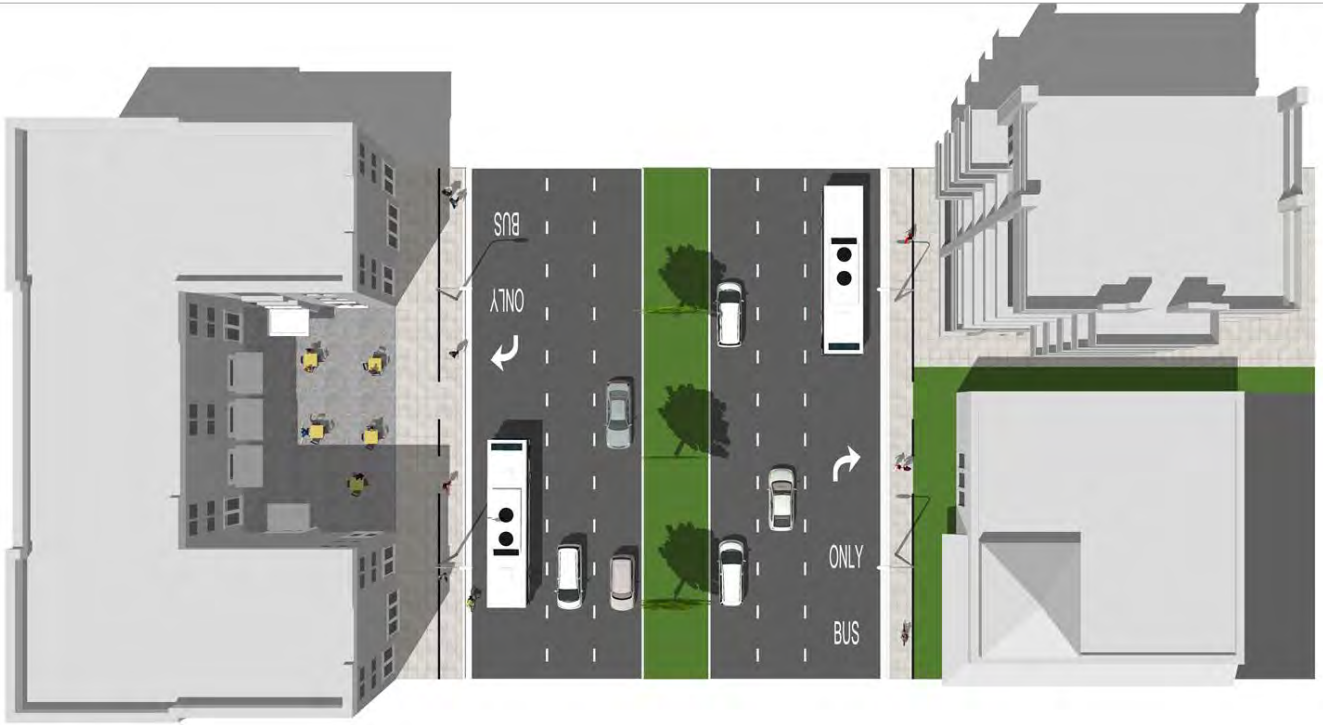
Figure 10: Alternative A aerial showing inconsistent sidewalk width
