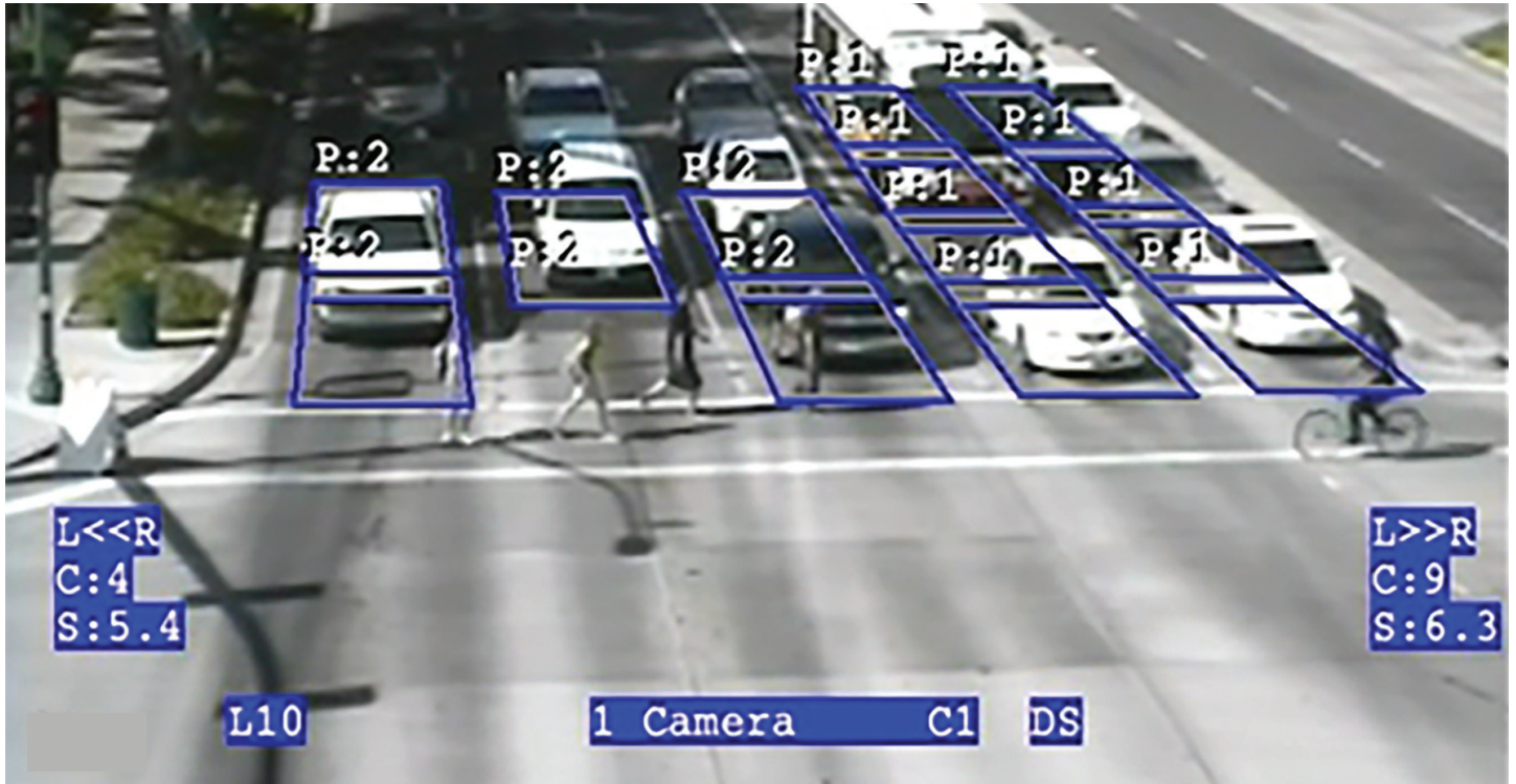
PedTrax data (shown in blue) for bi-directional counts and speeds of pedestrians moving left-to-right and right-to-left.
