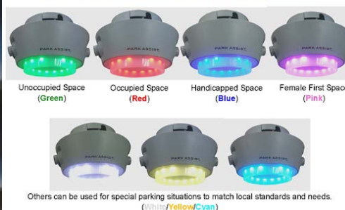
LED Status Indicators of M4 CAMERA SENSOR
