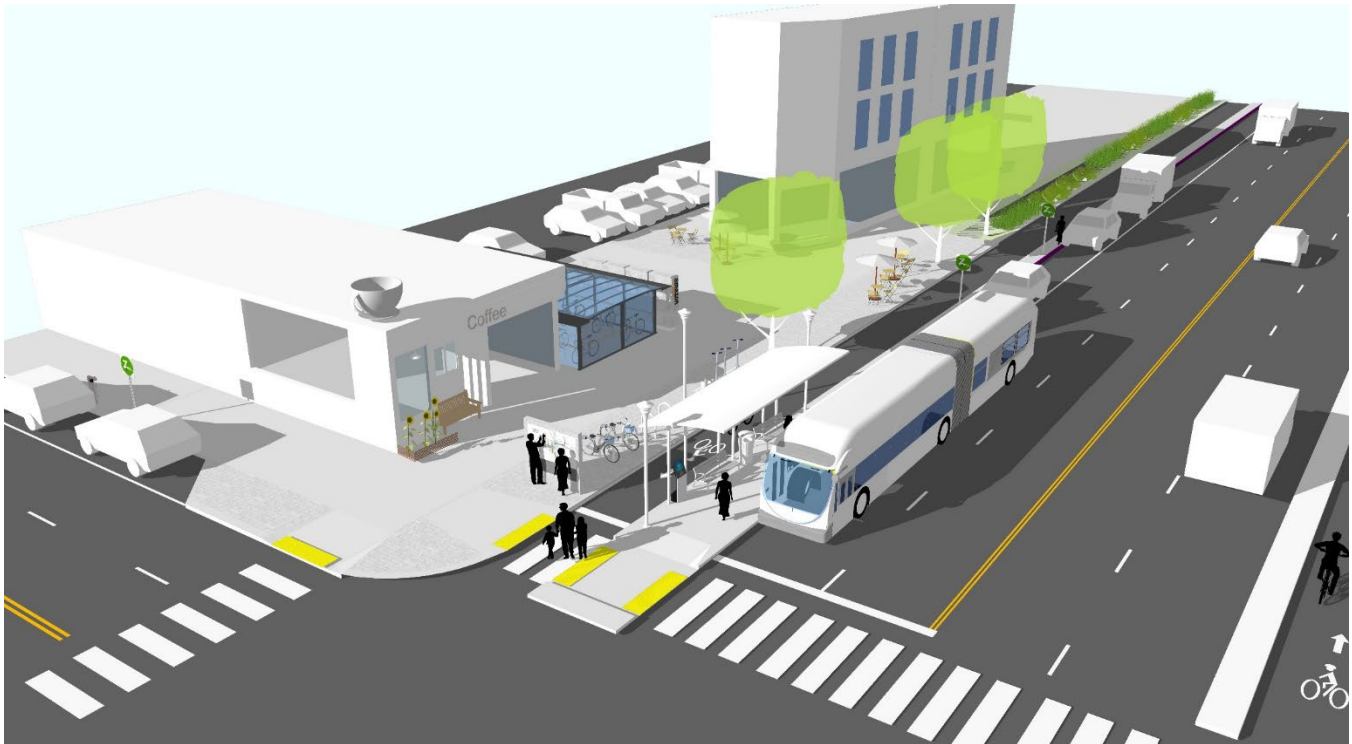
Figure 3. Example Midsize Mobility Hub with linkages to regional bus stops, micromobility, parking and local amenities.
