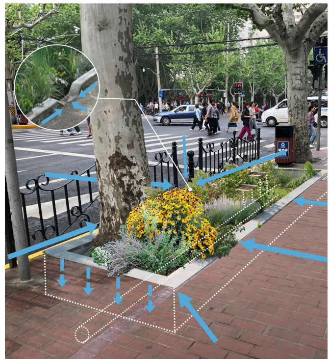
Example of a bioretention trench with trees and vegetation designed to capture, infiltrate, and release stormwater runoff from the sidewalk and a curb cut.
