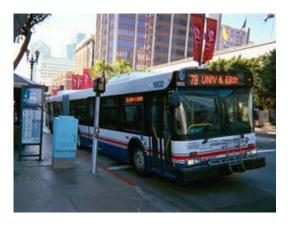
Figure 21. Sixty-foot long articulated buses provide higher capacity on busy arterial routes
