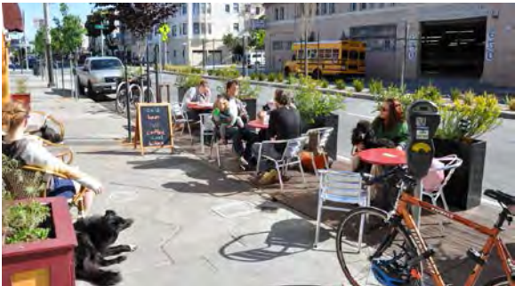
Parklets can extend the sidewalk by at least 8 feet providing space for seating and amenities
